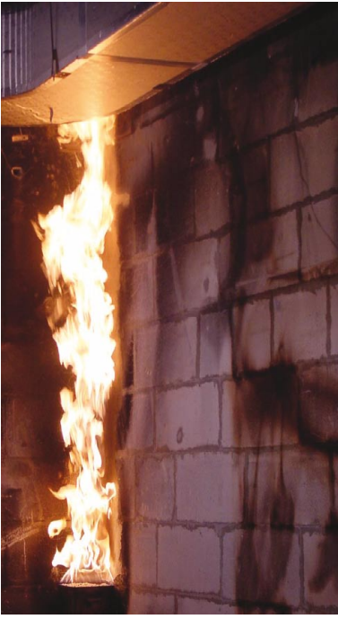
Fig. 9 - Simulation of a fire with the room corner test
