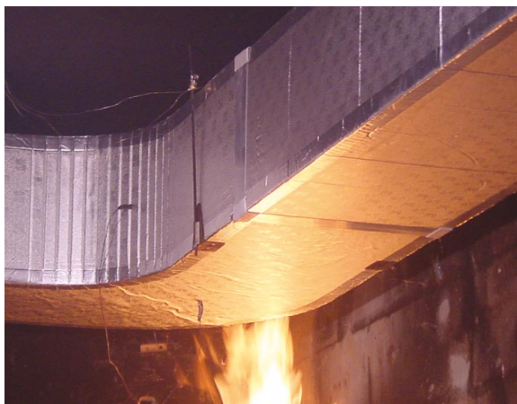
Fig. 14 - 100 kW thermal attack (development phase)
