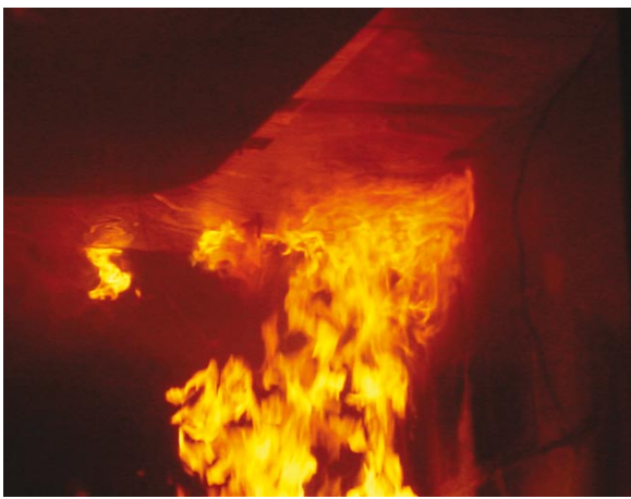
Fig. 15 - 300 kW thermal attack (generalised fire)
