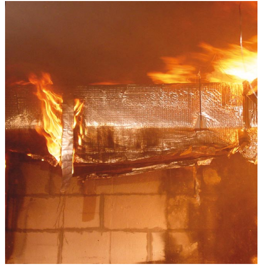
Fig. 17 -The metallic duct participates considerably to the fire propagation.
